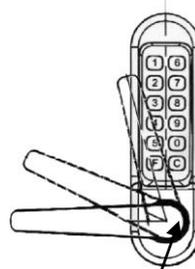
Locate the Grub Screw in the Lever Handle unscrew and remove it using the supplied Allen Key.
