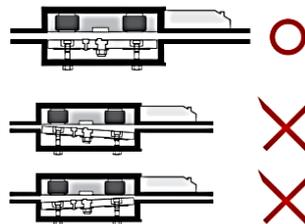
Make sure the gap between the Shear Lock and the Armature Plate are the same while adjusting the gap.
