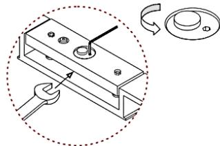
Use spanner and allen wrench to release the Locking Bolt on the Armature Plate. Rotate the position of the Locking Bolt in order to correctly seat inside the keep hole of the Shear Lock.
